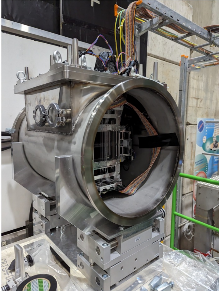
(a) UTS with SFH prototype in the target area. (b) Gel pad used to improve the SiPM-fiber coupling in the SFH prototype.
