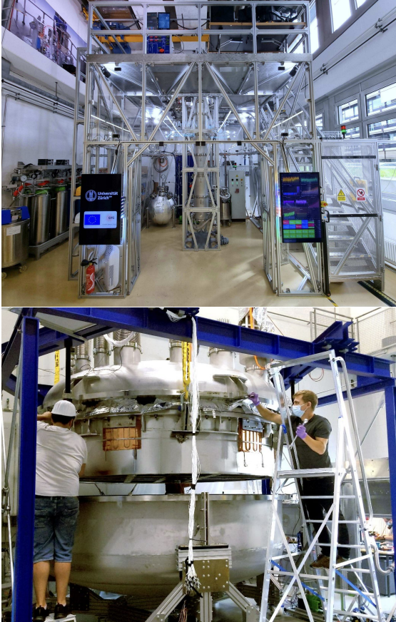
Figure 7: Pictures of the large-scale DARWIN R&D facilities Xenoscope, in Zurich (top), and Pancake, in Freiburg (bottom). Xenoscope (Baudis et al., 2021, 2023) will operate a 2.6 m tall TPC inside the 3.5 m tall cryostat, while Pancake will test 2.6 diameter electrodes as well as a 2.6 diameter TPC.
